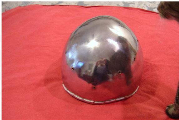
I first started by removing the rivets and smoothing the holes left. For decorative effect, I used some thin brass grommets to fill in the holes left by the rivets.
